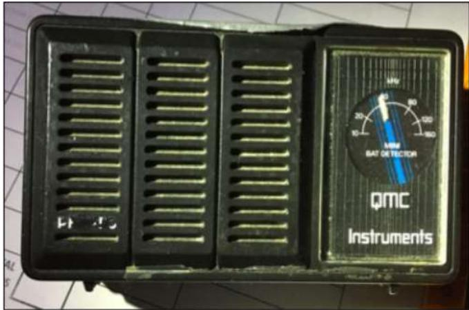
Figure 3. An image of one of the QMC bat acoustic detectors used throughout the project. (V. Caron, 2018).
