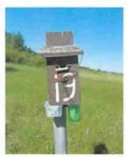
A Tree Swallow box equipped with a perch counter, RFID detector, and iButton temperature recorders
