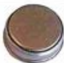
An ibutton; the device inserted into Tree Swallow nests to record temperature at regular intervals
